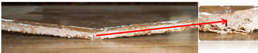
Figure 7. Matrix crack observed in composite specimen
